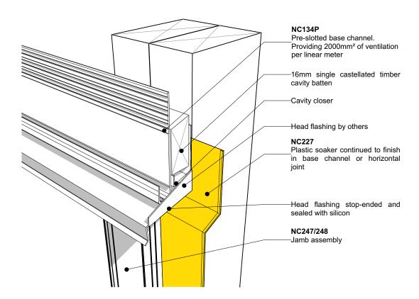
Junction after cladding around window head
