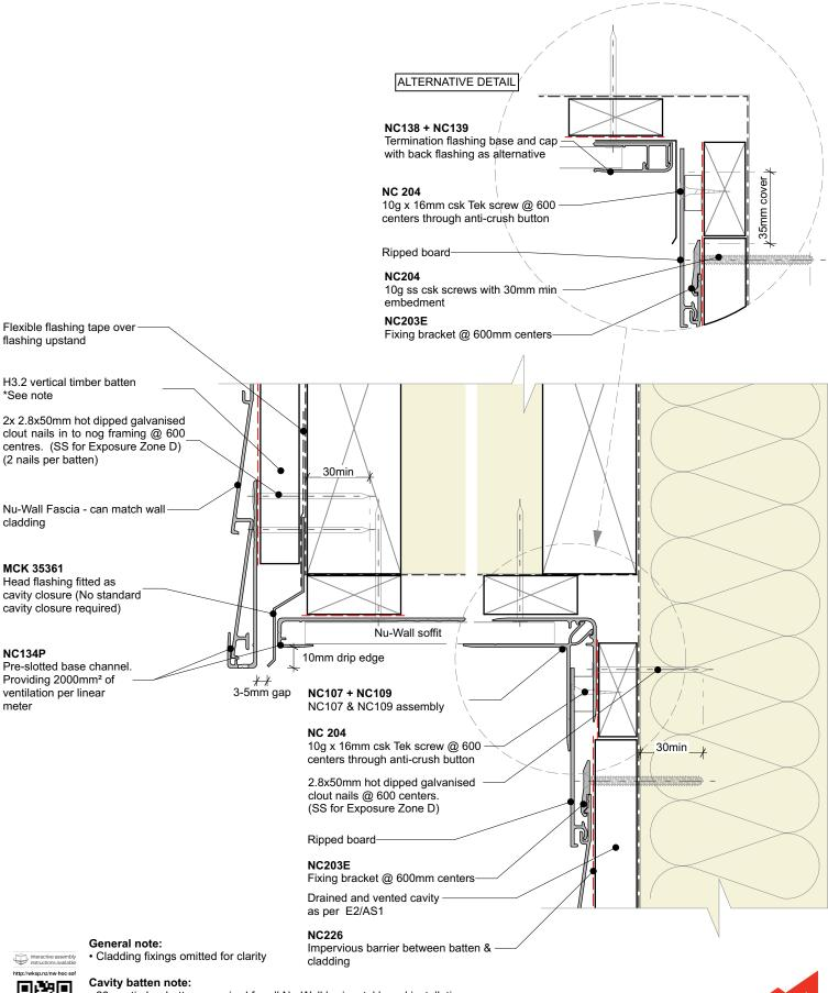
20mm timber battens required for all Nu-Wall horizontal board installations
